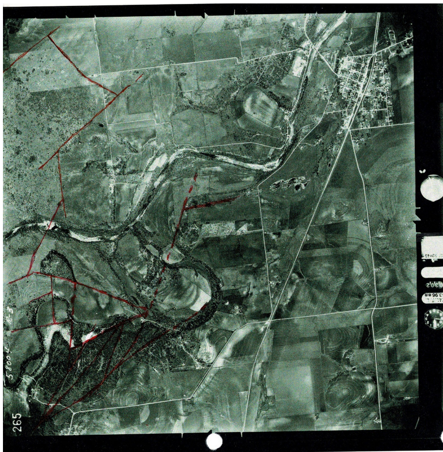
Figure 8. Preliminary Photogeologic Map of the Balcones Fault Zone Area around the MBML. The dashed fault across the meander loop separates the Del Rio Clay (and perhaps the Buda Limestone) on the northwest side of the fault from the Austin Chalk in the cut bank on the southeast side.
