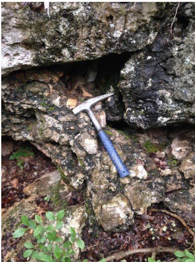
Closer View of Outcrop, Showing Possible Fault Gouge as Conglomerate. Photo Courtesy of Brian Hunt.
