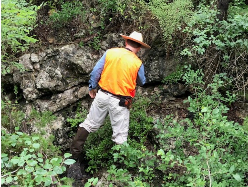
Outcrop Showing Beds That Are Dipping Into the Bank of the Small Stream. Brian Is Examining the Fault Evidence
