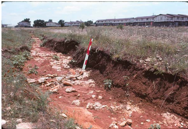
Figure 4-14. Channel Scour Attributed to Urbanization
