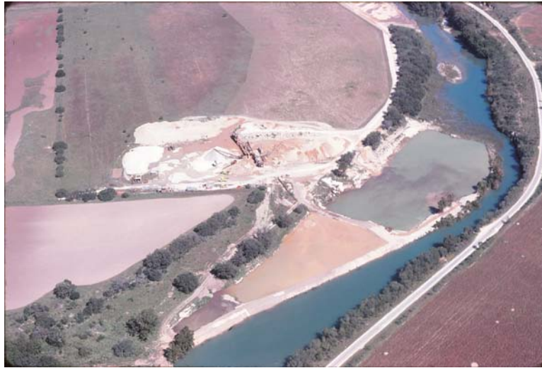
Figure 4-17. Wet-operation Sand and Gravel Pits
